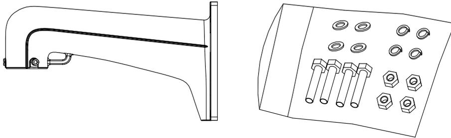
Figure 2-5 Wall Mount Bracket, Nuts and Flat Washers
