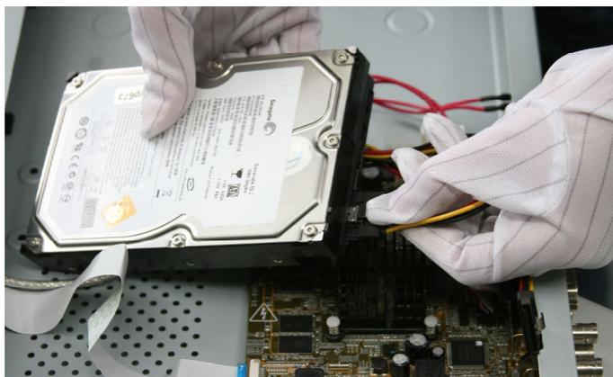
Figure 2. 4 Connect Power Cable
