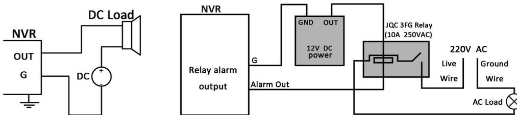
Figure 2. 7 Alarm Output Wiring
