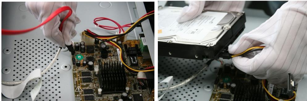
Figure 2. 3 Connect Data Cable
