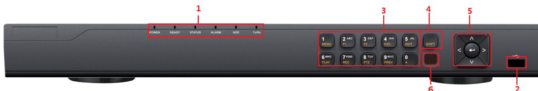
Front Panel of 16ch-FT/FA and 8ch-ST series
