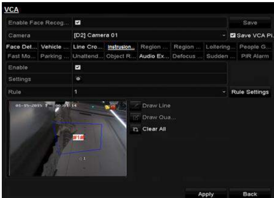
Figure 9-5 Draw Area for Intrusion Detection
