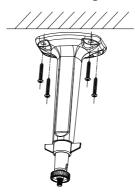
2.2. Install the camera to the bracket with the supplied screws.
