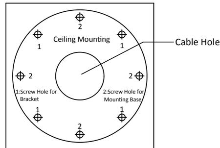
3. Fix the camera to the wall/ceiling with the supplied screws
