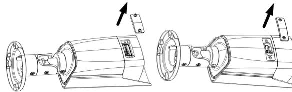
2) Insert the memory card into the memory card slot
