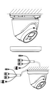
Rotate the camera horizontally from 0° to 30° as shown below until it is adjusted to the best viewing angle, then tighten the locking screw.
