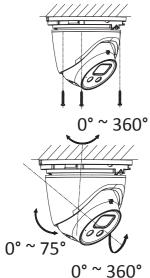
Before installation, loosen one Pan locking screw.
