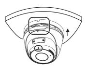
Adjust the housing to the position shown in figure above. Align the screw hole on the housing with the tail cable outlet on the base, attach the housing gently and then rotate clock/counterclockwise at least 8 degrees to lock. To ensure proper image display and illumination effects, make sure the mark (see figure above) is aligned with the screw hole when installation is complete.
