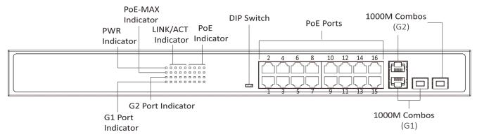
Figure 1-1 POE-SW1602N Front Panel
