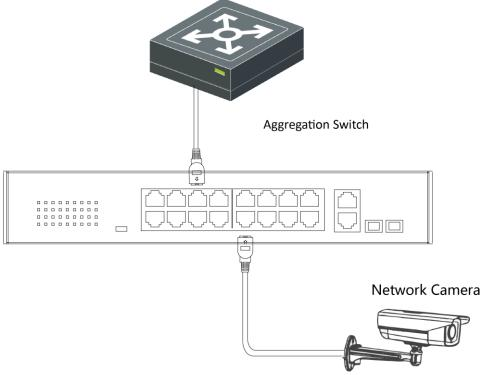
Figure 3-1 RJ45 Port Connection
