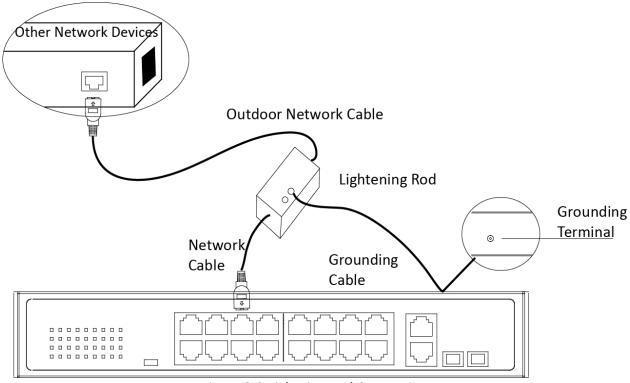
Figure 3-2 Lightning Rod Connection
