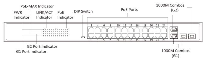
Figure 1-2 POE-SW2402N Front Panel
