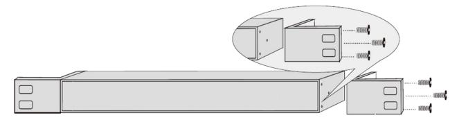
Figure 2-1 Install L-Shaped Bracket
