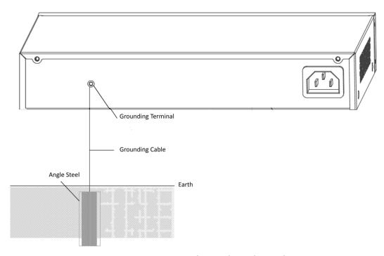
Figure 2-4 Grounding with Angle Steel
