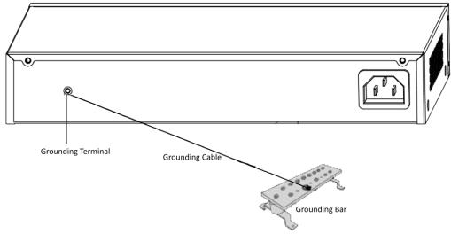
Figure 2-3 Grounding with Grounding Bar
