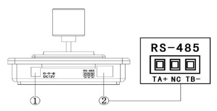
1、 Power input connector: input DC12V power.
