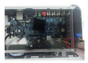
1. Pull the battery cable through the hole.
