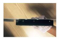
3. Put the HDD onto the bracket.
