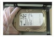
3. Put the HDD into the Device.
