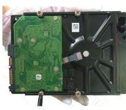
2. Fix the screws on the HDD, but do not be fastened.
