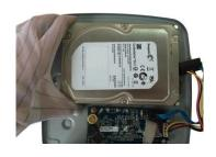
3. Match the screws with the holes on the DVR to place the HDD.
