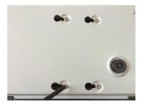
Turn the device to see the back side of it. Align the screws of the HDD with the holes on the back of the device, and then fix the screws.
