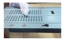
Match the holes on the bracket with the screw holes on HDD.
