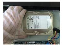
Place the HDD onto the Device.
