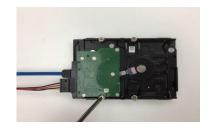
2. Connect HDD cable and power cable to HDD, and fasten the screws in HDD.
