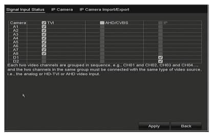
Figure 2-13 Configure Signal Input Type
