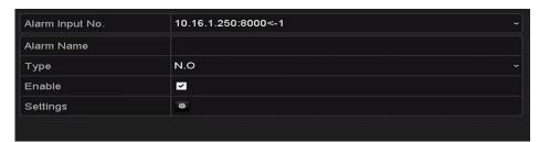
Figure 8-6 Alarm Input Settings Interface
