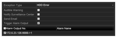
Figure 12-24 Configure HDD Error Alarm
