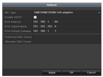
Figure 11-23 Network Parameters Configuration
