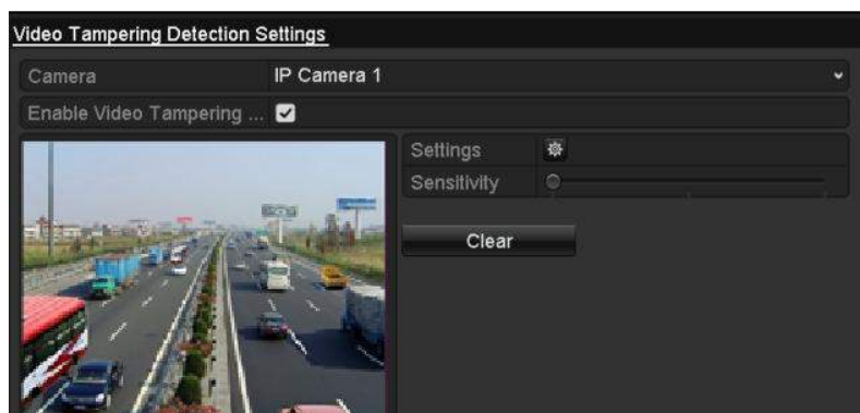
Figure 8. 11 Video Tampering Setting Interface
