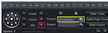
\* Select COC protocol in P.T.Z configuration interface and then call 95 Preset or click “Iris +” here to enable the menu of the camera which supports COC. Please refer to the user manual of the relevant camera for more details.
