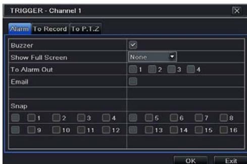
**Buzzer:** If selected, the local buzzer would be activated on an alarm.
