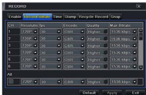
Set up rate, resolution, quality, encode and max bit stream according to the actual situation.
