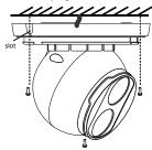
Mount your camera. Mount the housing with install mark aligned
