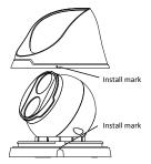
Install the base plate and the camera. Connect cable and protect it with waterproof tape and attach turret to ceiling with taping screws.
