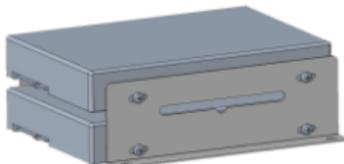
2. Fasten the brackets installed with hard disks to the device.
