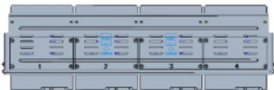
4. Put the mounting plate back in place. Connect the power cables and data cables as shown in the figure. Repeat the steps to connect all the disks.
