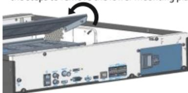
3. Secure the disks on the mounting plate. Fix the screws according to the figure below. Avoid damaging the disk in the process.
