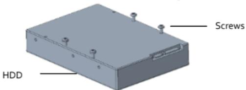
3. Slide the disk into place from A to B, and fix the screws to secure the hard disk.
