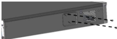
2. Turn the upper mounting plate in the shown direction, then remove the plate. Repeat the steps to remove the lower mounting plate (for 8-HDD devices only).
