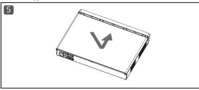
Screw the upper cover screws back on.
