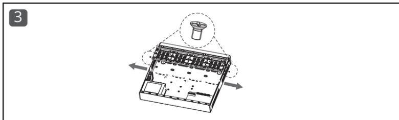
Align and screw the HDD to the bracket.
