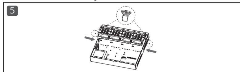
Connect the HDD's SATA and power cable to the device.
