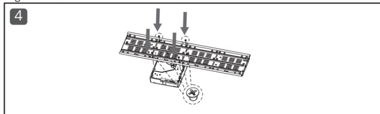
Install the bracket and HDD using the side screws.
