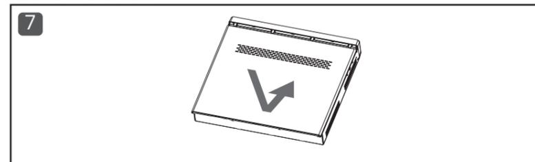
Screw the upper cover screws back on.
