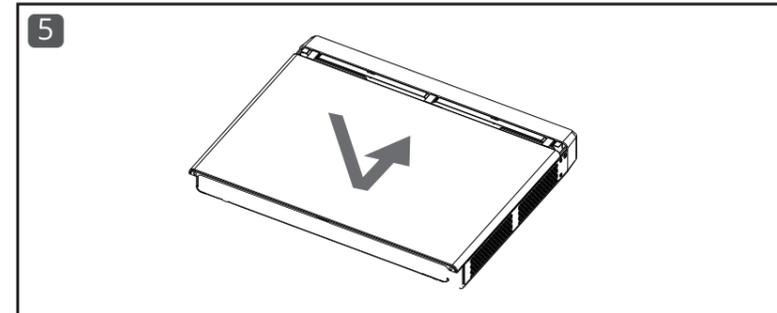
Screw the upper cover screws back on.
