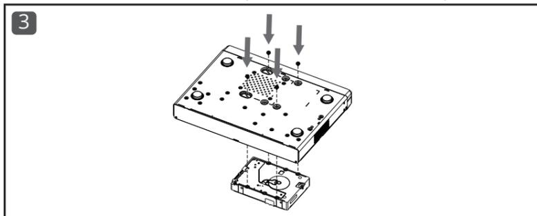
Connect the HDD's SATA and power cable to the device.
