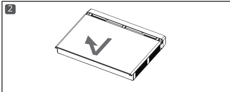
Turn the device over. Use the screws provided to secure the HDD in place.
