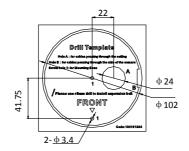
Align the screw holes and cable hole on the drill template and the base plate, and then fix the base plate to the ceiling with the two supplied screws.
