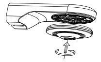
Re-install the main body of the bracket to the mounting base, and fix it with the screw.
