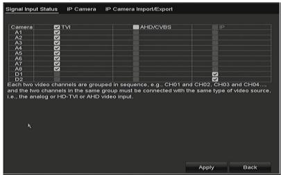
Figure 3. 6 Configure Signal Input Type
