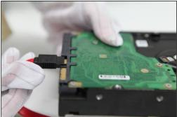
Figure 2. 2 Connect the Data Cable
