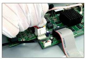
Figure 2. 3 Connect the Power Cable
