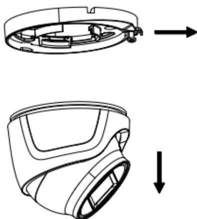
Figure 2-19 Remove the Mounting Base
