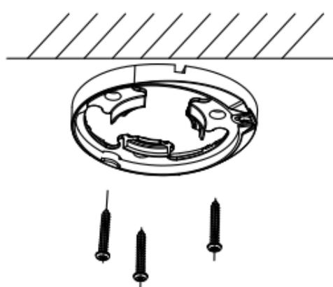
Figure 2-20 Secure the Mounting Base to the Ceiling
