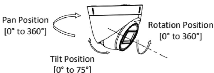
Figure 2-6 3-Axis Adjustment
