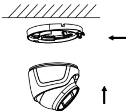
Figure 2-21 Secure the Camera
