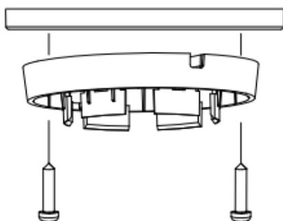
Figure 2-16 Install the Mounting Base
