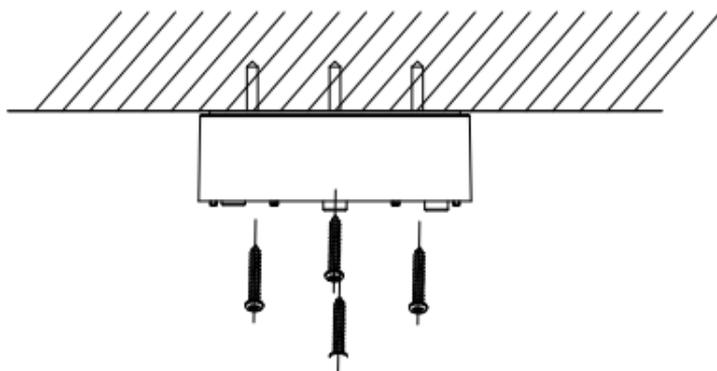
Figure 2-17 Secure the Junction Box's Body
