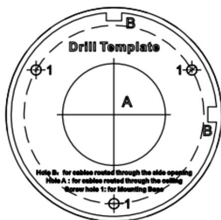
Figure 2-15 The Drill Template
