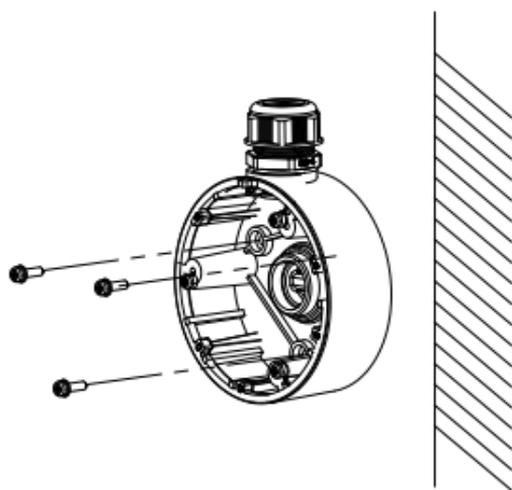
Figure 2-8 Secure the Junction Box
