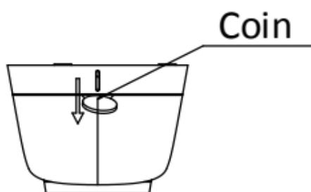
Figure 2-2 Pry the Mounting Base
