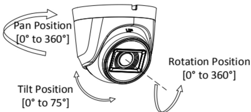
Figure 2-14 3-Axis Adjustment
