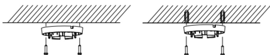
Figure 2-12 Attach the Mounting Base
