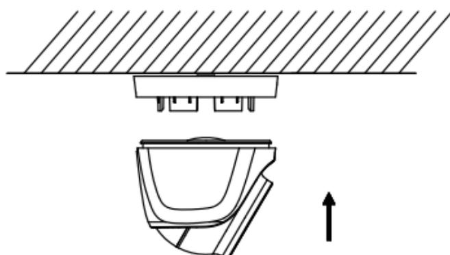
Figure 2-13 Install the Camera Back
