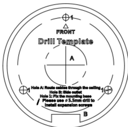
Figure 2-7 The Drill Template
