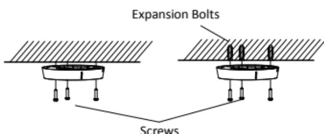
Figure 2-4 Attach the Mounting Base to the Ceiling
