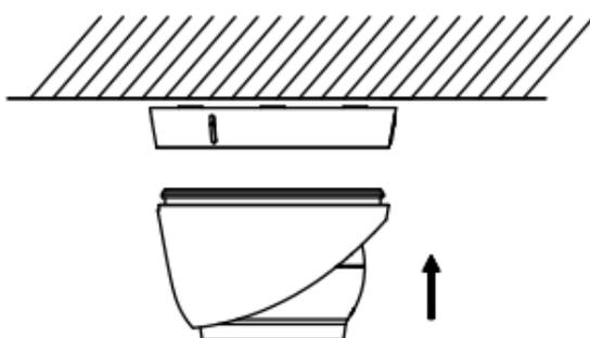
Figure 2-5 Install the Camera Back
