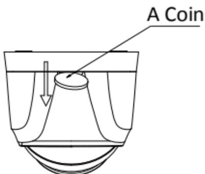
Figure 2-10 Pry the Mounting Base
