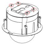
Figure 2-6 Remove 4 screws
