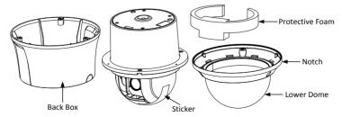
Figure 2-14 Disassemble the Speed Dome
