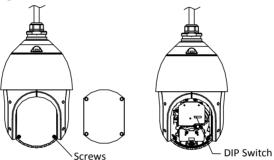
Figure 1-7 DIP Switch of Mini IR Speed Dome
