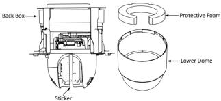
Figure 2-1 Remove the Protective Accessory
