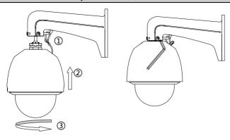
Figure 1-15 Install the Speed Dome
