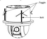
Figure 2-15 Install the Toggle Bolts
