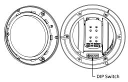
Figure 1-2 DIP Switch of Mini Analog Speed Dome
