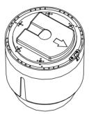
Figure 2-7 Remove the in-ceiling mounting mount
