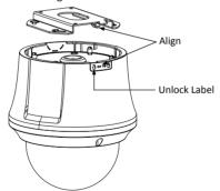
Figure 2-22 Install Speed Dome
