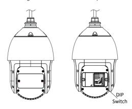
Figure 1-8 DIP Switch of 5-inch IR Speed Dome
