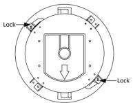
Figure 2-3 Locks and Lock Screws
