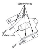
Figure 2-11 Secure the Mounting Base
