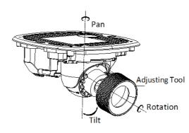
9. Tighten the hex screw to fix the well-adjusted surveillance angle.
