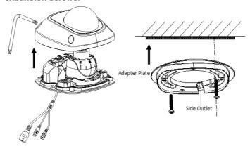
4. Fix the dome drive with the supplied screws.
