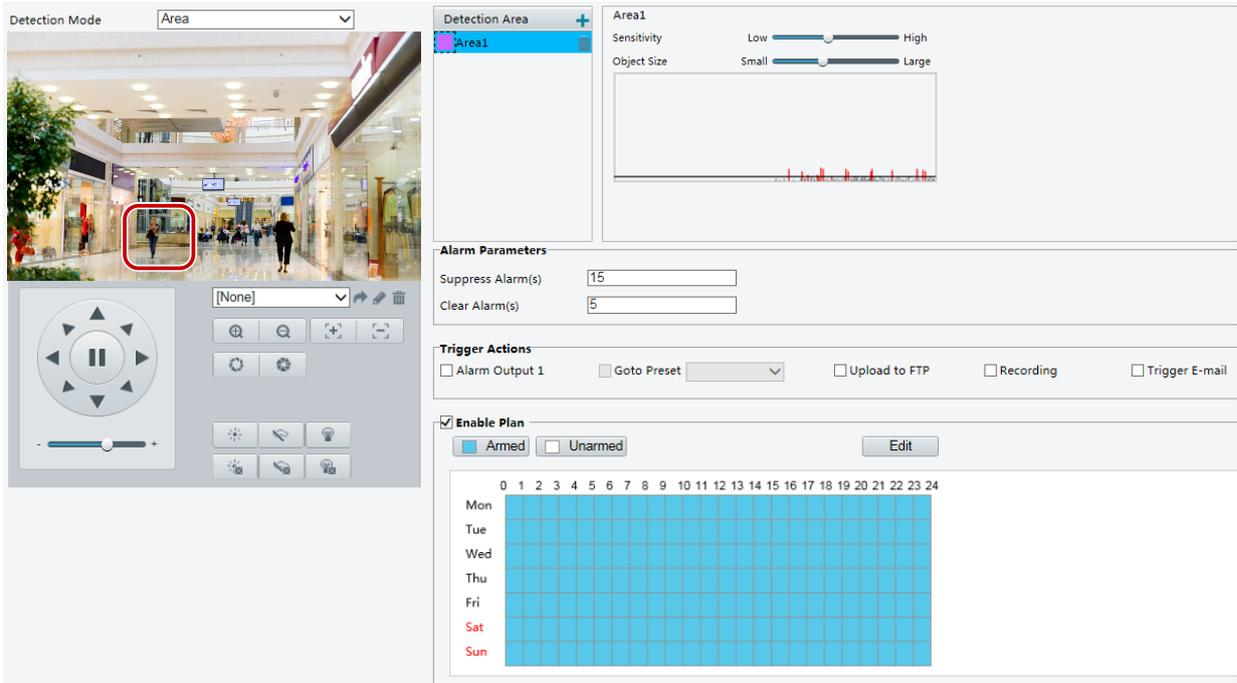
2. In the **Detection Area** area, click
