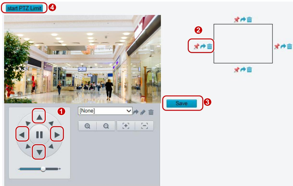
2. Use directional buttons to rotate the camera to an intended position.
