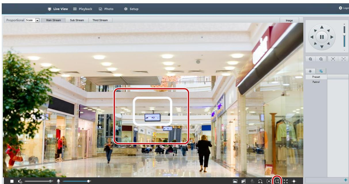
2. Click and hold the mouse button, and then drag from top down (draw a rectangle) to specify an area. Dragging reversely (from down top) will zoom out.
