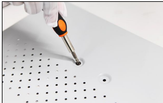
Figure 2. 4 Install the HDD
