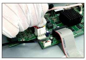
Figure 2. 3 Connect the Power Cable
