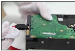
Figure 2. 2 Connect the Data Cable
