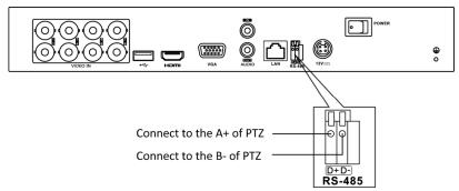
Figure 2. 5 Controller Connection A
