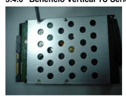
①Use 4 screws to secure the HDD
