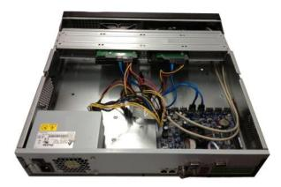
3 Connect to the HDD data cable to the main board and the HDD port respectively. Loosen the power cable of the chassis and connect another end of the power cable to the HDD port.
