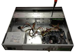
① Use the screwdriver to loose the screws of the rear panel and then remove the front cover.
