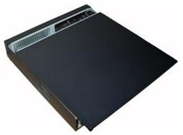
$\textcircled{4} \quad \text{After connect the cable, put the front cover back to} \quad$ the device and then fix screws of the rear panel.
