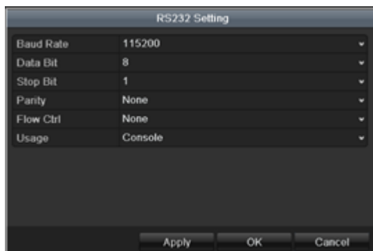
Figure 14. 7 RS232-Receive port Settings Interface
