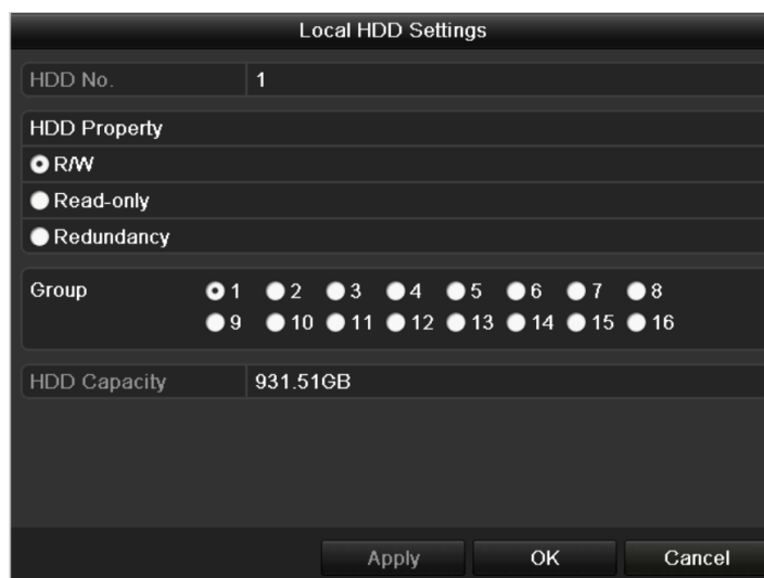
Figure 11. 15 Local HDD Settings Interface
