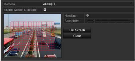
Figure 8. 2 Set Detection Area and Sensitivity
