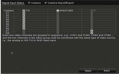
Figure 2. 16 Configure Signal Input Type
