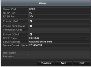
Figure 2. 7 Advanced Network Parameters
