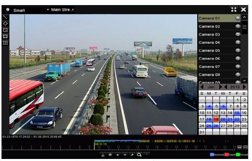
Figure 6. 9 Smart Playback Interface
