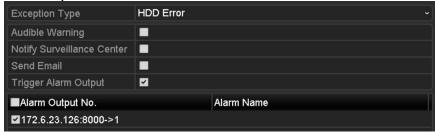
Figure 13. 23 Configure HDD Error Alarm
