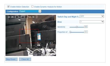
Figure 5-8 Motion Detection Settings-Expert
