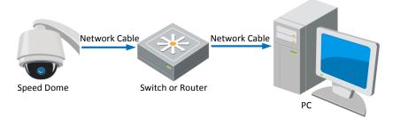
Figure 2-2 Connecting via a Switch or a Router
