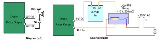
Figure A.10.1 Alarm Out Connections
