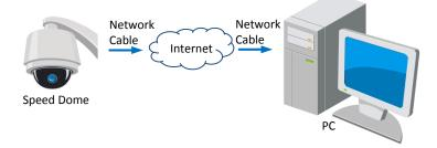
Figure 2-11 Accessing the Speed Dome with Static IP Directly
