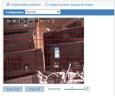
Figure 5-7 Motion Detection Settings-Normal
