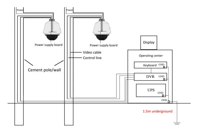
Figure A.3.2 Grounding in Cement Pole/Wall Installation
