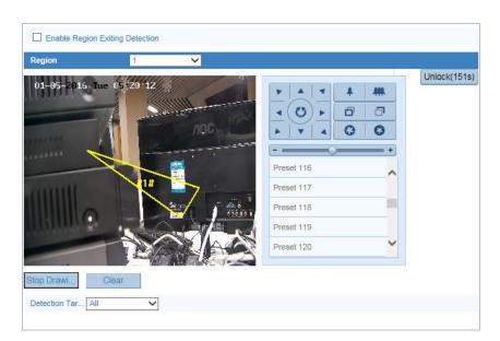
Figure 5-23 Configuring Region Exiting Detection
