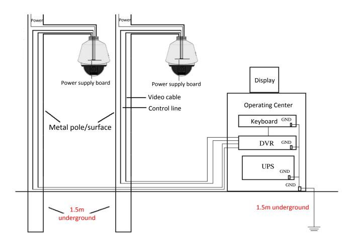
Figure A.3.4 Grounding in Metal Pole Installation
