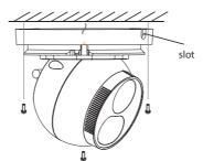
5. Mount your camera. Mount the housing with install mark aligned.
