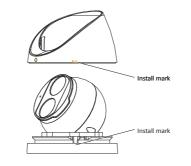
4. Install the base plate and the camera. Connect cable and protect it with waterproof tape and attach dome to ceiling with taping screws.
