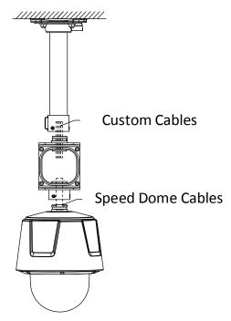
Figure 3-84 Assemble the Speed Dome with Bracket
