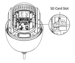
Figure 2-14 Micro SD Card Slot
