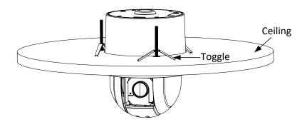
Figure 2-25 Install the Dome to the Ceiling
