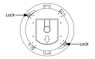
Figure 3-43 Locks and Lock Screws
