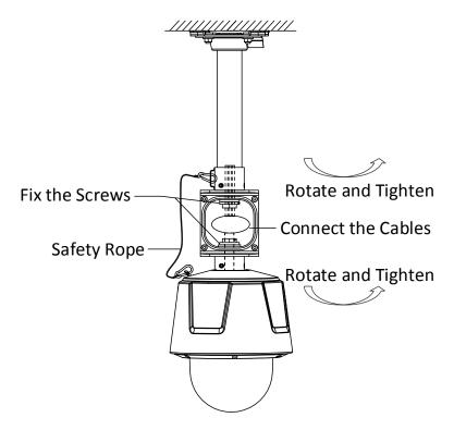
Figure 3-86 Fix the Screws and Connect the Cables 9) Connect the corresponding cables inside the gang box.
