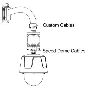
Figure 3-68 Assemble the Type II Gang Box and the Bracket
