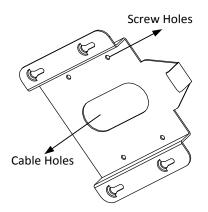
Figure 3-49 Mark the Screw Positions
