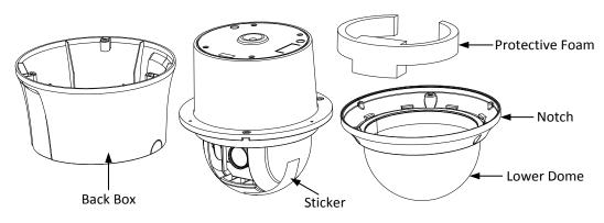
Figure 2-22 Disassemble the Speed Dome
