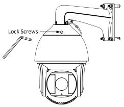
Figure 3-32 Secure the Speed Dome
