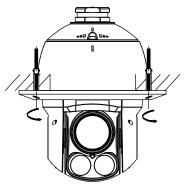
Figure 2-30 Install the Dome to the Ceiling
