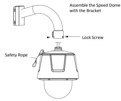
Figure 3-57 Assemble the Speed Dome with Bracket
