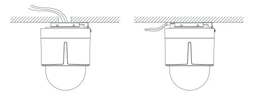
Figure 2-43 Cabling for Ceiling Mounting
