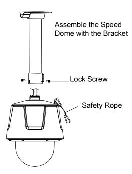
Figure 3-74 Assemble the Speed Dome with Bracket
