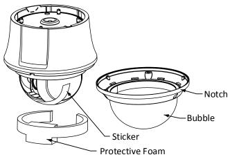
Figure 2-37 Disassemble the Speed Dome
