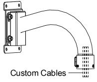
Figure 3-67 Getting the Cables through the Bracket
