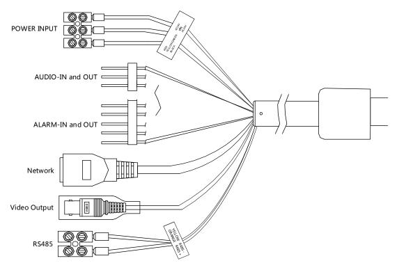
Figure 2-3 Cables of Network Speed Dome
