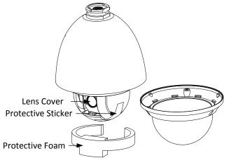
Figure 2-7 Remove the Protective Accessories
