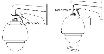
Figure 3-9 Install the Speed Dome
