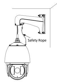
Figure 3-22 Install the Speed Dome
