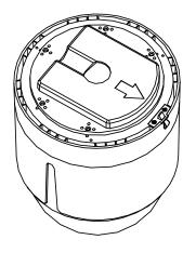
Figure 2-41 Remove the Bracket
