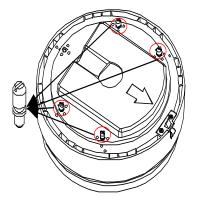
Figure 3-47 Install the Bolts
