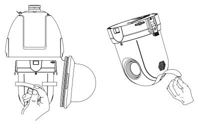
Figure 3-4 Remove the sticker for Integrated 5-inch speed dome
