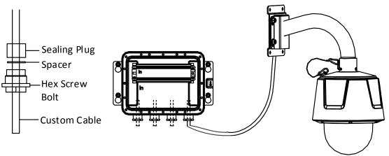
Figure 3-63 Connect the Cable 4) Fix the cover with screws to accomplish the installation.
