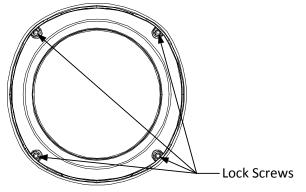
Figure 3-12 Loosen the Lock Screws
