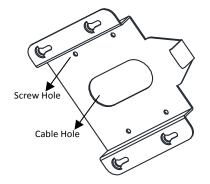
Figure 2-44 Mark the Screw Positions
