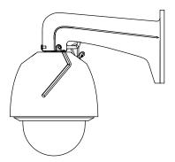
Figure 3-10 Secure the Speed Dome
