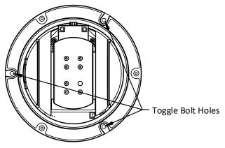
Figure 2-23 Toggle Bolt Holes
