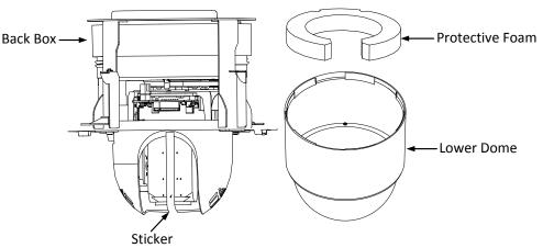
Figure 2-32 Remove the Protective Accessory
