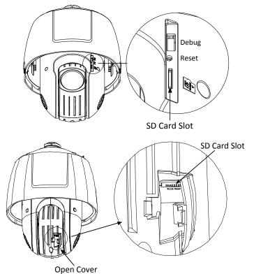
Figure 3-14 Install the SD Card
