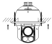
Figure 2-29 Push to the Mounting Hole
