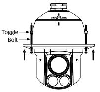
Figure 2-28 Install Toggle Bolts
