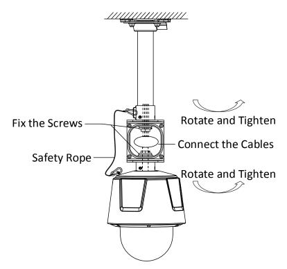
Figure 3-70 Fix the Screws and Connect the Cables 5) Connect the corresponding cables inside the gang box.
