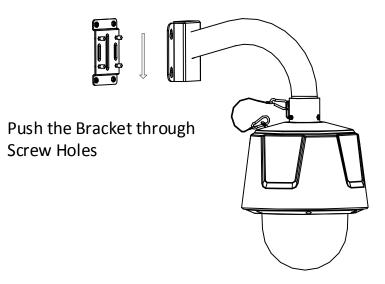
Figure 3-60 Install the Speed Dome
