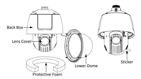
Figure 3-13 Remove the Protective Elements
