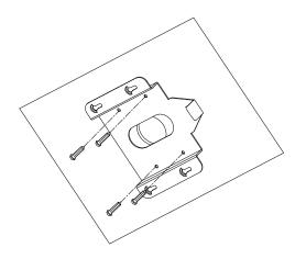
Figure 3-50 Secure the Mounting Base
