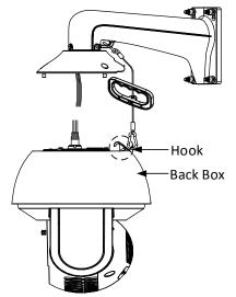
Figure 3-30 Hang the Speed Dome
