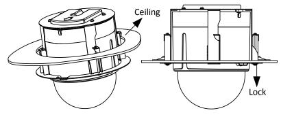
Figure 3-44 Install the back box
