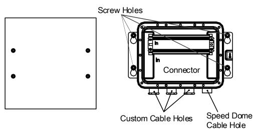
Figure 3-78 Install the Gang Box Type I
