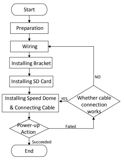
Figure 3-1 Installation Flow
