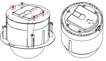
Figure 3-46 Remove the Bracket
