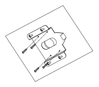
Figure 2-45 Secure the Mounting Base
