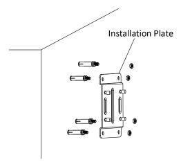
Figure 3-56 Attach the Installation Plate
