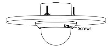
Figure 2-26 Install the Lower Dome
