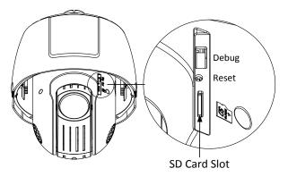
Figure 3-54 Install the SD Card
