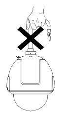
Figure 3-2 Do not Drag the Cables
