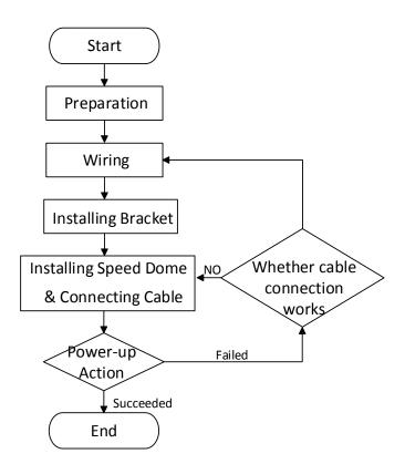
Figure 2-1 Installation Flow
