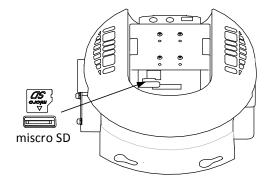
Figure 2-12 Micro SD Card Slot
