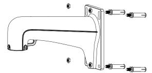
Figure 3-21 Install the Bracket
