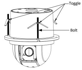
Figure 2-24 Install the Toggle Bolts
