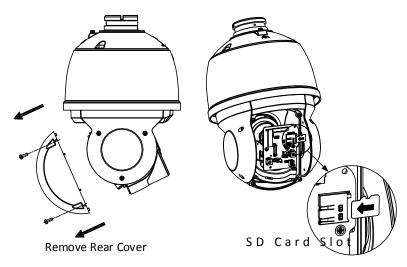
Figure 2-9 Micro SD Card Slot (Mini IR Speed Dome Type 1)
