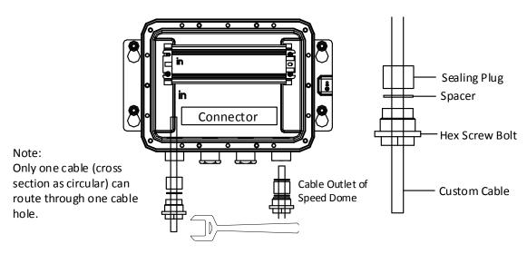
Figure 3-55 Interface of Custom Cables
