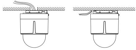
Figure 3-48 Cabling for Ceiling Mounting
