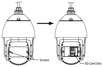
Figure 2-13 SD Card Slot
