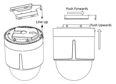
Figure 3-51 Attach the Back Box to the Mounting Base
