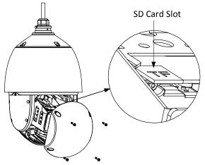
Figure 2-15 Micro SD Card Slot
