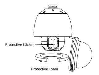
Figure 2-11 Remove the Protective Accessories
