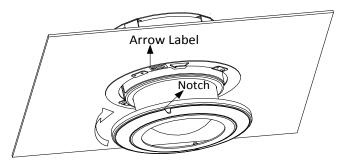
Figure 3-45 Install the Flange
