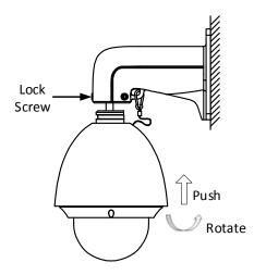
Figure 2-17 Align to the Bracket
