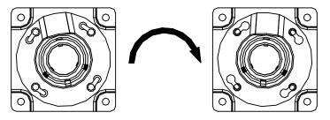
Figure 3-76 Fix the Installation Plate
