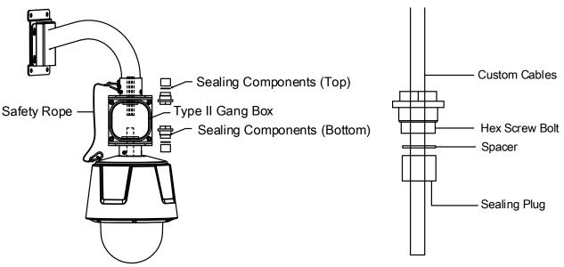
Figure 3-69 Assemble the Type II Gang Box with the Speed Dome
