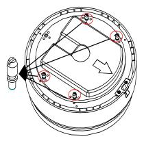
Figure 2-42 Install the Bolts
