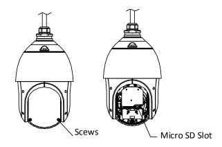
Figure 2-10 Micro SD Card Slot (Mini IR Speed Dome Type 2)
