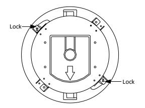
Figure 2-33 Locks and Lock Screws
