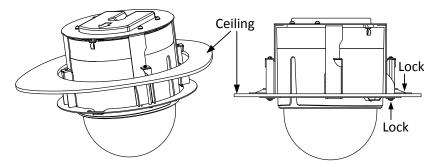
Figure 2-34 Install the back box
