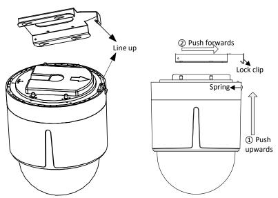
Figure 2-46 Attach the Back Box to the Mounting Base
