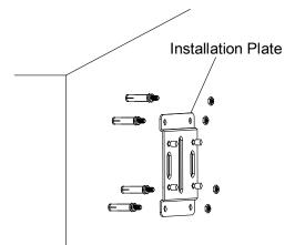
Figure 3-65 Attach the Installation Plate
