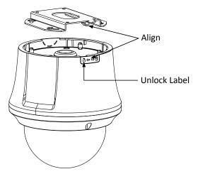
Figure 2-39 Install Speed Dome
