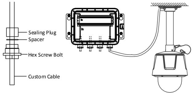
Figure 3-79 Connect the Cable
