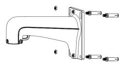
Figure 3-8 Install the Bracket
