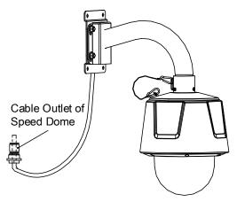
Figure 3-61 Fix the Speed Dome
