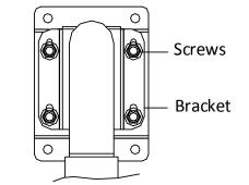
Figure 3-59 Fix the Installation Plate
