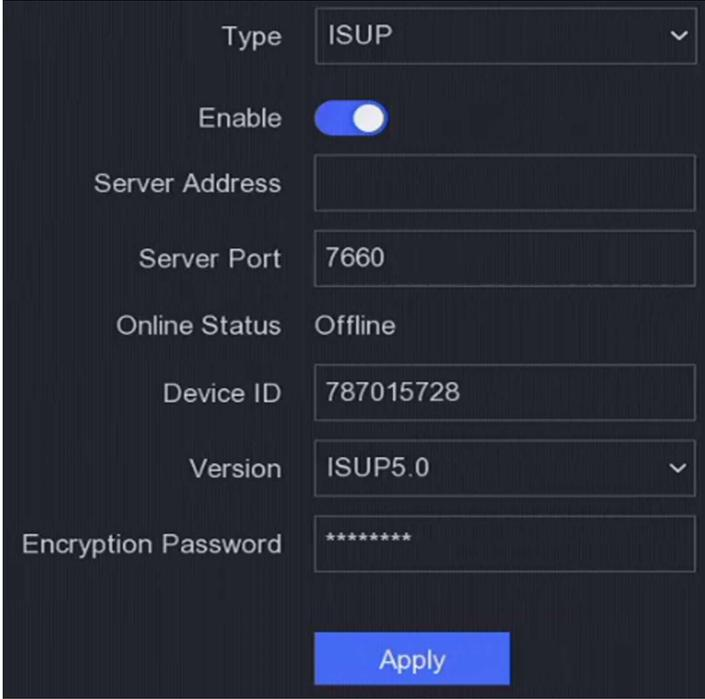
The screenshot shows a configuration window for ISUP. The 'Type' dropdown is set to 'ISUP'. The 'Enable' toggle is turned on. The 'Server Address' field is empty. The 'Server Port' field contains '7660'. The 'Online Status' is 'Offline'. The 'Device ID' field contains '787015728'. The 'Version' dropdown is set to 'ISUP5.0'. The 'Encryption Password' field contains '\*\*\*\*\*'. An 'Apply' button is at the bottom.
