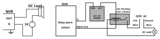
Figure 2. 7 Alarm Output Wiring
