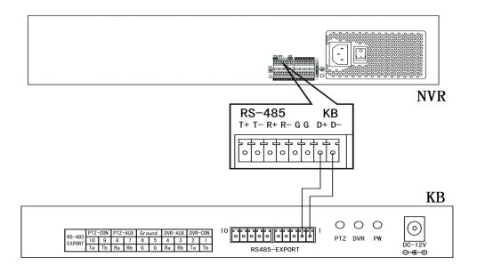
Figure 2. 8 Controller Connection
