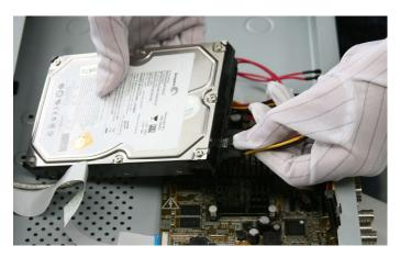
Figure 2. 4 Connect Power Cable
