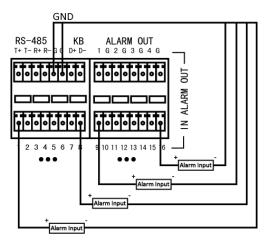
Figure 2. 6 Alarm Input Wiring
