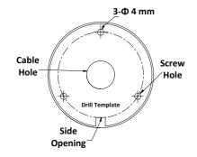
3. Route the cables through the cable hole (optional), or the side opening.
