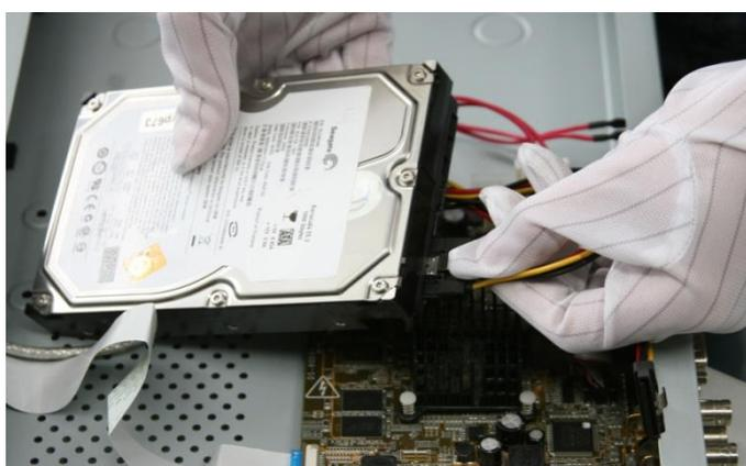
Figure 2. 3 Connect the power cable
