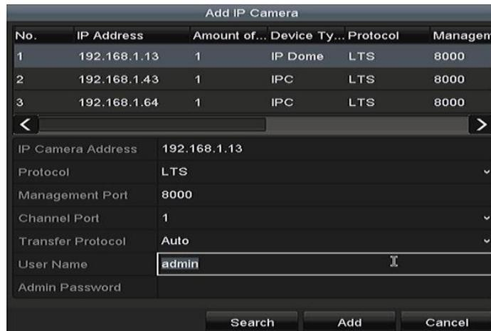
3. Select the detected IP camera and click the **Add** button to add it directly, and you can click the **Search** button to refresh the online IP camera manually.
