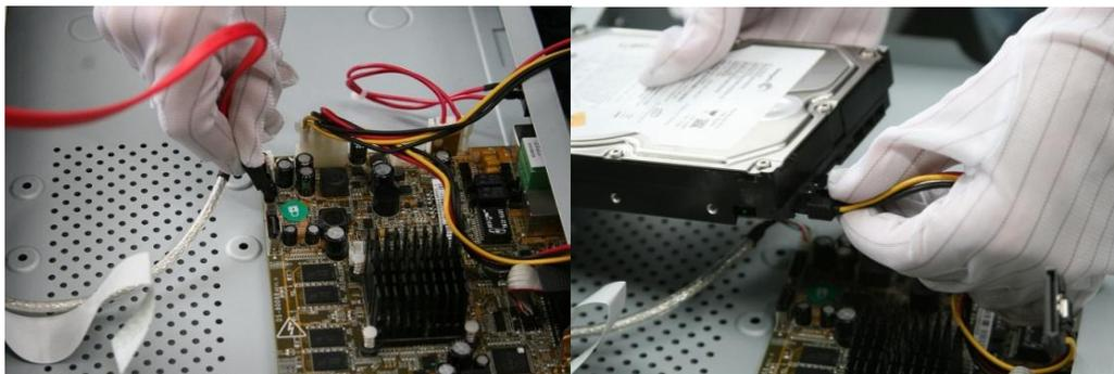
Figure 2. 2 Connect the data cable
