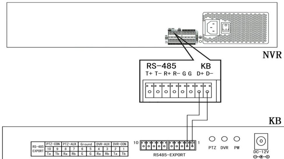
Figure 2. 6 Controller Connection
