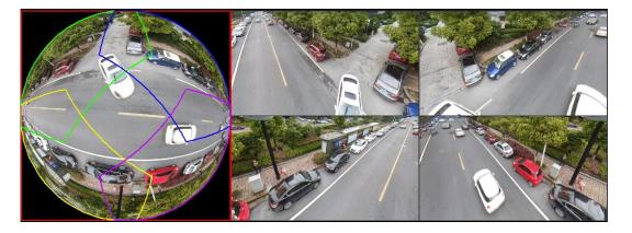
In Figure 4-75, you can adjust the color pane on the left pane or use your mouse to change the position of the small images on the right pane to realize fish eye de-warp.
