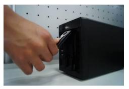
3Pull the HDD knob up when you put the HDD into the box in case the knob buckle may strike the front panel.
