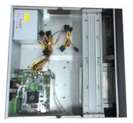
⑦ Put the bracket back. Please adjust the CD-ROM to the proper position so that the button of the front panel is directly facing the pop-up button of the CD-ROM.
