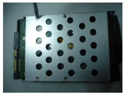
1 Use 4 screws to secure the HDD
