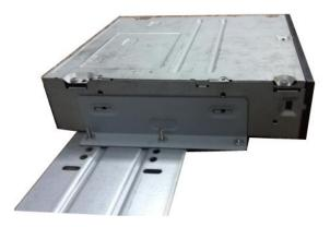
⑤ Install SATA burner. Line up the SATA burner to the hole positions.
