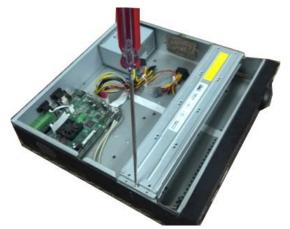
① Open top cover and then remove the HDD bracket
