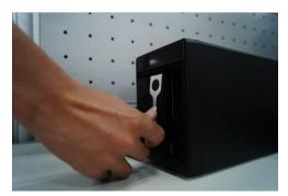
4 Put the knob back after you insert the HDD
