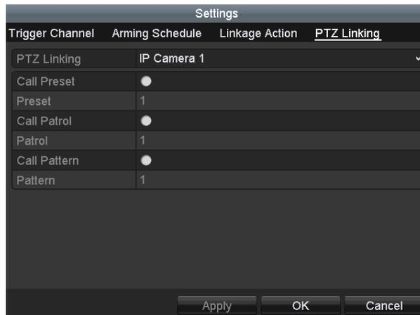
Figure 8. 6 Set PTZ Linking of Alarm Input
