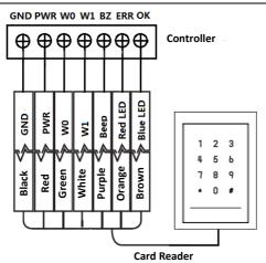
Figure 2-5 Wiring for Wiegand Communication Mode
