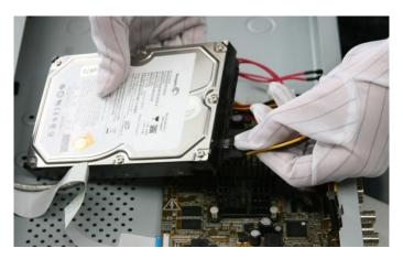
Figure 2. 3 Connect the power cable
