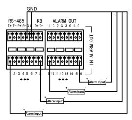
Figure 2. 4 Alarm Input Wiring
