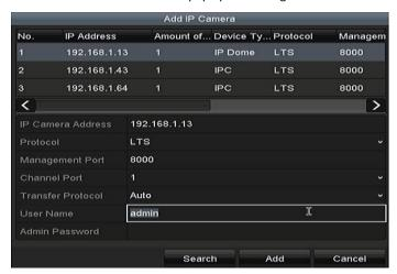
**3.** Select the detected IP camera and click the **Add** button to add it directly, and you can click the **Search** button to refresh the online IP camera manually.
