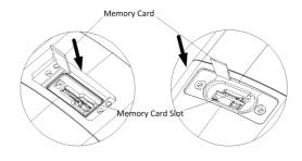
3)(Optional)To unmount the memory card, push to get it ejected4)Screw the cover back to the camera
