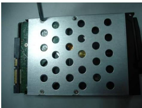
① Use 4 screws to secure the HDD
