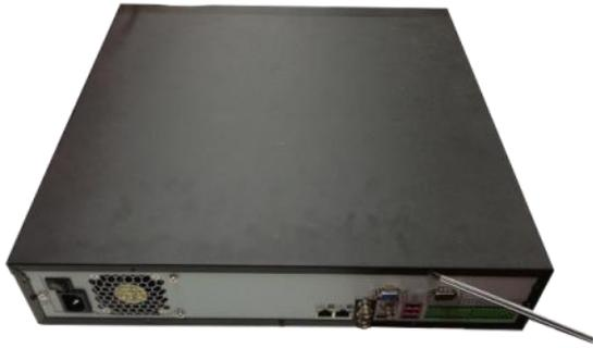
① Use the screwdriver to loose the screws of the rear panel and then remove the front cover.
