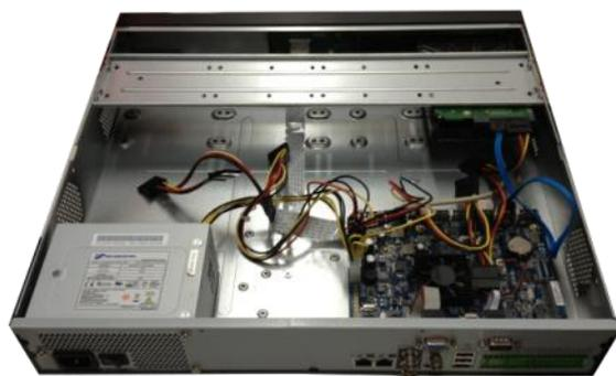
③ Connect to the HDD data cable to the main board and the HDD port respectively. Loosen the power cable of the chassis and connect another end of the power cable to the HDD port.
