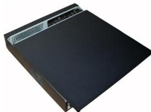
④ After connect the cable, put the front cover back to the device and then fix screws of the rear panel.
