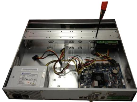
① Use the screwdriver to loose the screws of the rear panel and then remove the front cover.
