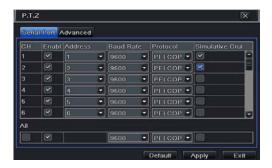
[Address]: The address of the PTZ device.
