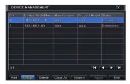
You may also select the added device and click "Setup" button to modify channel, IP address of the device.
