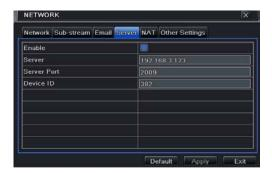
④ Input the above-mentioned server IP, server port and device ID in the server interface. Then click "Apply" button to save the setting. Now, the ECMS/NVMS system will automatically connect this device.
