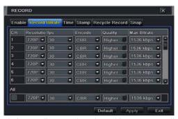
Set up rate, resolution, quality, encode and max bit stream according to the actual situation.
