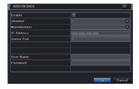
**Note**: If the HD TVI Hybrid DVR and the IP cameras you want to add are in WAN, the IP address of the IP camera input here must be WAN IP.
