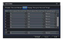
**Expiration Time:** Set the expiration time for recorded video. If the set date is overdue, the recorded files will be deleted automatically.
