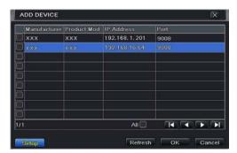
If the IPC is not in the same local network, you can select the device and click "Setup" to modify the IP address of the searched device.
