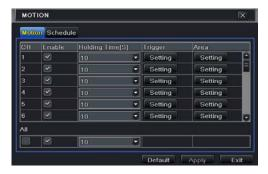
③ Go to alarm handling setting by click "Setting" button under Trigger. Then go to "To Record" tab. You can select the recording channel and click "OK" button to confirm the settings.
