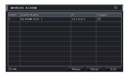
Choose alarm out and click "Alarm" button to trigger alarm manually. Click "Clear" button to clear the alarm.
