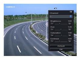
② In this interface, you can adjust brightness, hue, saturation and contrast in live. Click "OK" button to save the setting.
