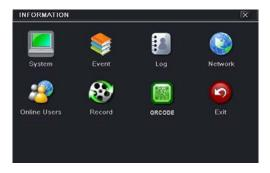
Click "System" to check the hardware version, MCU version, kernel version, device ID, etc.
