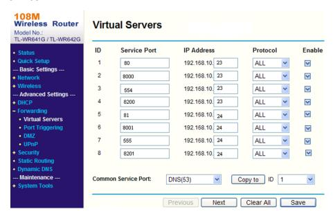
Figure 7-1 Port Mapping on Router
