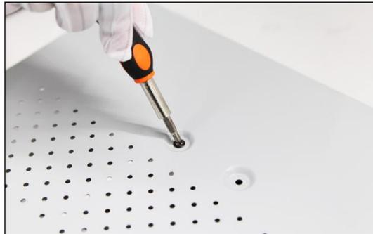
Figure 2. 4 Install the HDD
