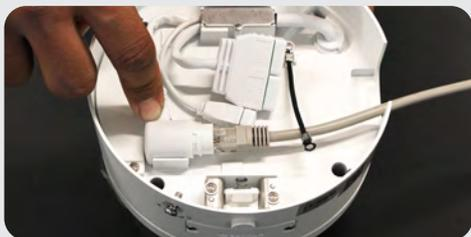
The InstaDome has a removable plate that comes off, revealing neatly arranged cables within the junction box, significantly reducing installation times by 80%.
