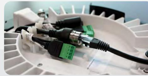
We are significantly reducing labor costs by utilizing a single PoE (Power over Ethernet) cable to support a camera with five lenses. This approach eliminates the need for five separate cables and cameras, streamlining installation and maintenance while improving efficiency.
