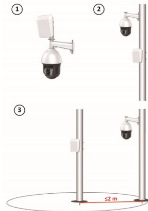
Figure 10-18 Scenario of One-Point Calibration
