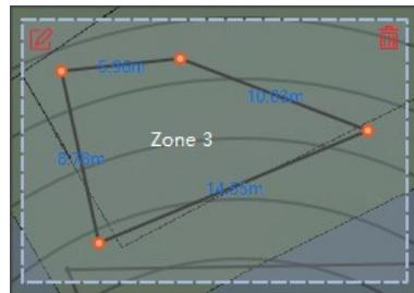
**Figure 10-17 Point Cloud Filter Zone**
