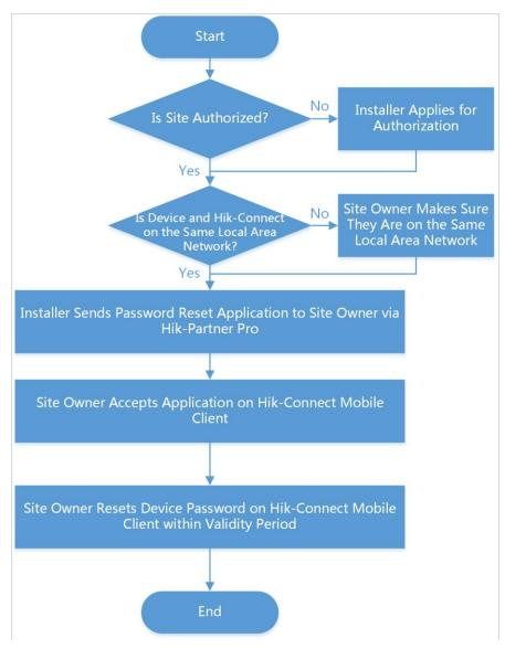
Figure 7-7 Flow Chart of Resetting Device Password Offsite
